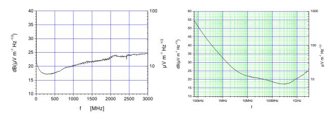
Probe Sensitivity (Noise Equivalent Field Strength) (typ.)
